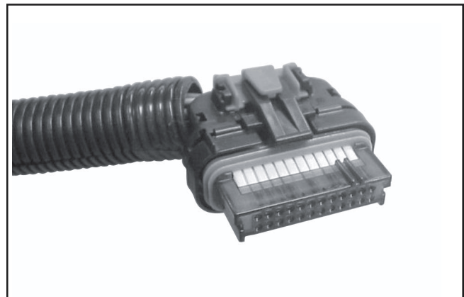
Figure 5B-23. 24 Pin Connector (Plastic-Cased ECU).
