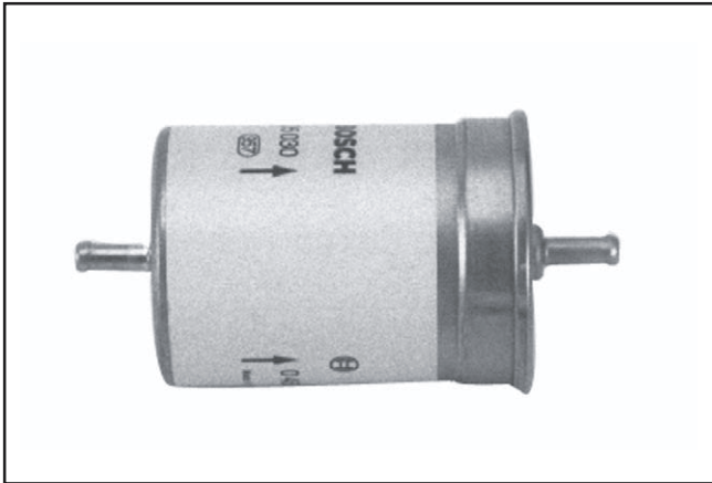
Figure 5B-28. In-Line Fuel Filter.
