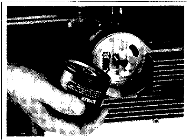
Figure 11-81. Installing New Oil Filter.
