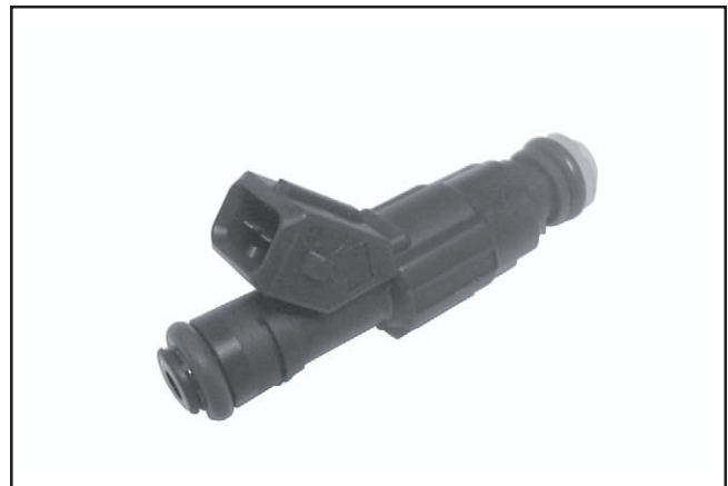
Figure 5B-16. Style 2 Fuel Injector.
