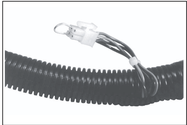
Figure 5B-7. Service Connector Plug, Metal-Cased ECU Harness.
