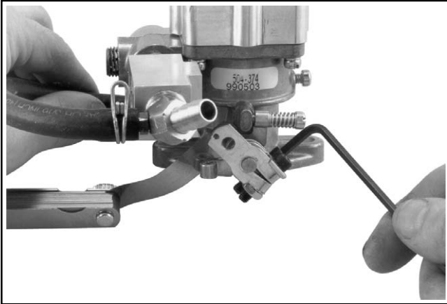
Figure 5A-10. Tightening Idle Speed Clamp Mounting Screw.
