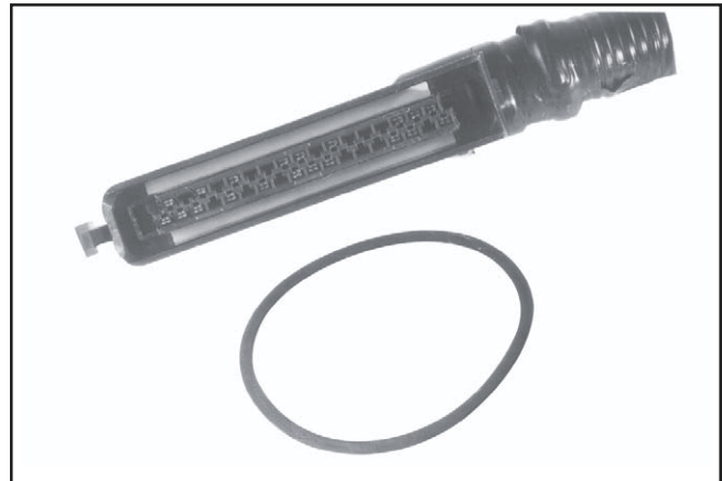
Figure 5B-22. 35 Pin Connector and O-Ring (Metal-Cased ECU).
