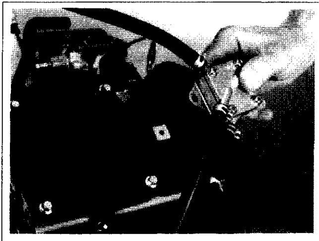
Figure 9-15. Remove Fuel Pump and Lines as an Assembly.
