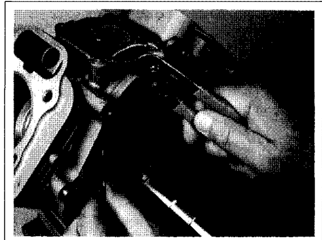
Figure 11-4. Installing Governor Cross Shaft Hitch Pin.
